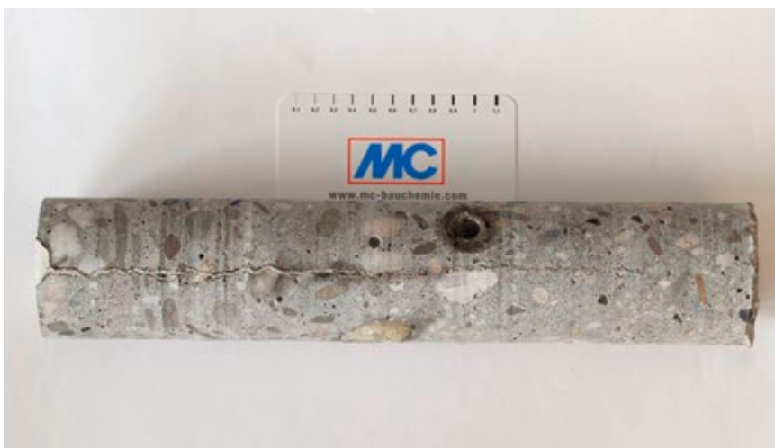
This section through an injected component clearly shows the depth of penetration achieved through even the finest of hairline cracks with MC-Injekt 2133 flex
